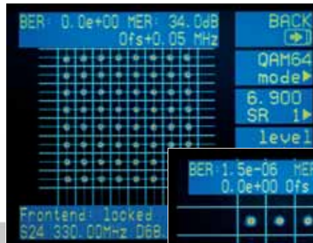
Constellation diagram of a QAM64 signal
