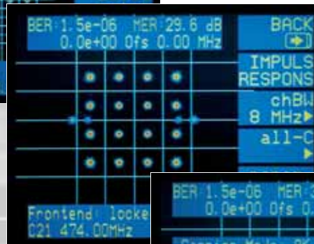
Constellation diagram of an OFDM signal (16QAM)
