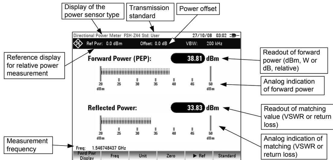
The power sensors contain frequency-dependent correction values. This means that the highest accuracy is reached for signals whose frequency is known. When the R&S FSH switches to the power measurement mode from another operating mode, it transfers its current center frequency to the power sensor.
