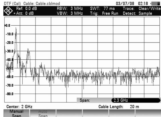
The minimum span that can be set is either 1/10 of the span automatically set by the R&S FSH in the case of AUTO SPAN or 200 MHz (whichever is smaller). Spans larger than the ones set by the R&S FSH with AUTO SPAN are not allowed.
