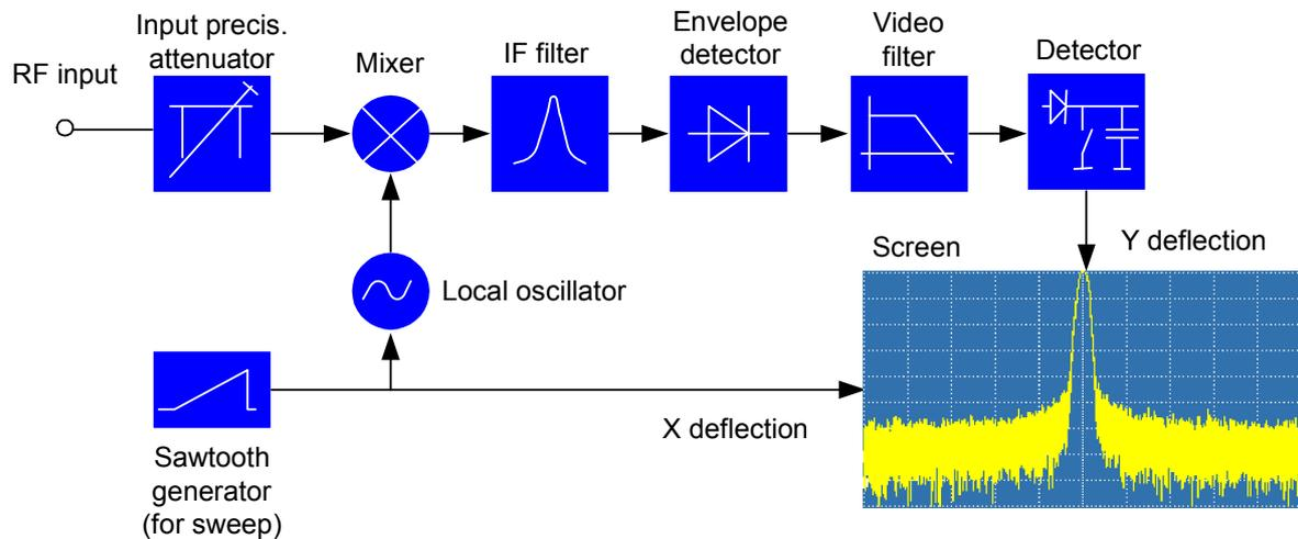
The precision attenuator at the input of the spectrum analyzer adjusts the level of the measurement signal to the level range that the mixer can handle without overdriving it. The precision attenuator at the input of the R&S FSH is adjustable in 10 dB steps from 0 dB to 30 dB and is directly coupled to the reference level setting.
