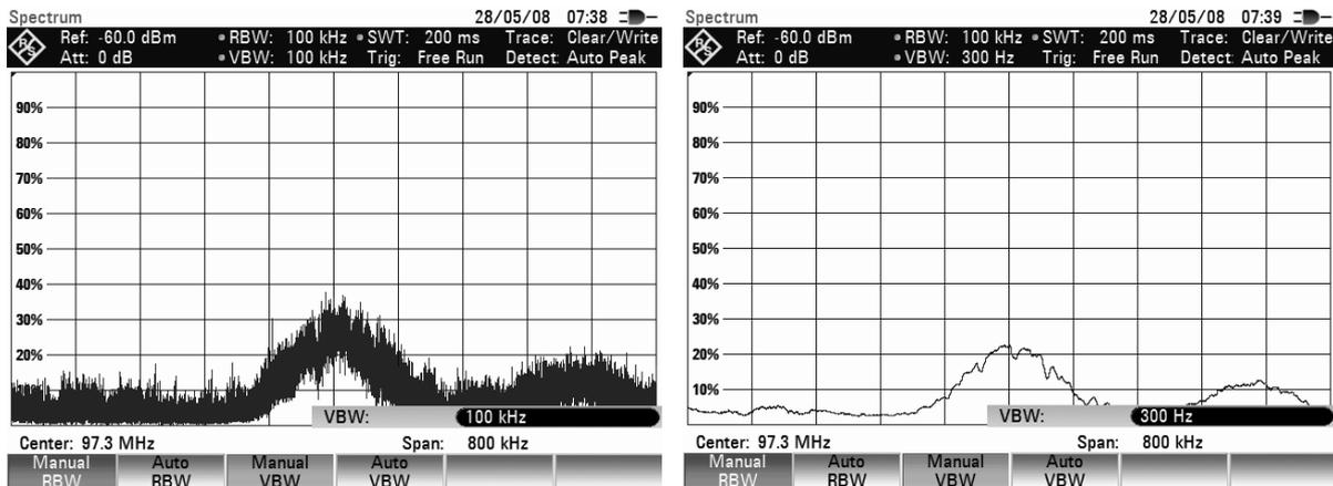
Limiting the video bandwidth smoothes the trace considerably. This makes it much easier to determine the level of the measured signal.
