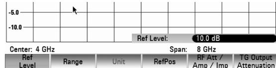
When performing measurements on amplifiers, make sure the R&S FSH is not overdriven. The risk of overdriving is eliminated when the trace is within the display area on the screen (with REF POSITION = 10 dB).
