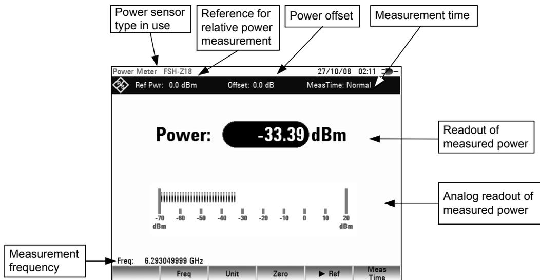
The power sensor has a memory containing frequency-dependent correction values. This means that the highest accuracy is reached for signals whose frequency is known. If the R&S FSH switches over to the power measurement mode from another operating mode, it uses the center frequency as the frequency for the power sensor.
