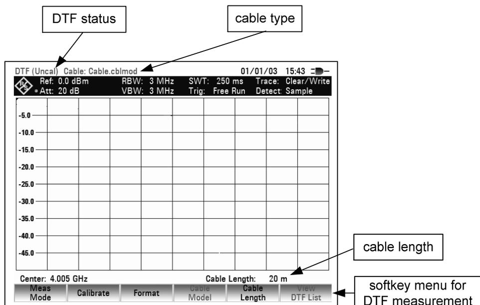
To perform distance-to-fault measurements, the R&S FSH needs to “know” the type of cable and its approximate length.
