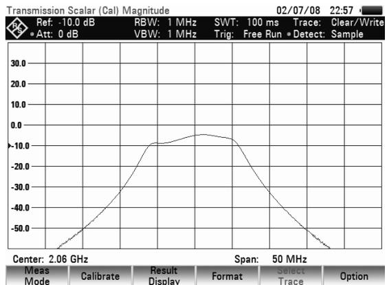
The transmission calibration remains valid until the center frequency or the span is changed on the R&S FSH to such an extent that the new span falls outside the calibrated frequency range. UNCAL is displayed in the upper area of the screen when calibration is no longer valid.
