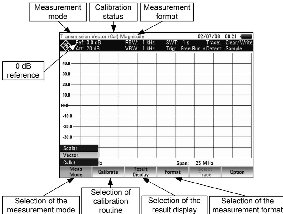
When the tracking generator is switched on, the status display indicates UNCAL. This indicates that tracking generator measurements are uncalibrated. The level axis is in the relative unit dB. Apart from the level values, the 0 dB reference is also displayed. This corresponds to a reference level of 0 dBm in the spectrum analyzer mode (= nominal output level of the tracking generator).
