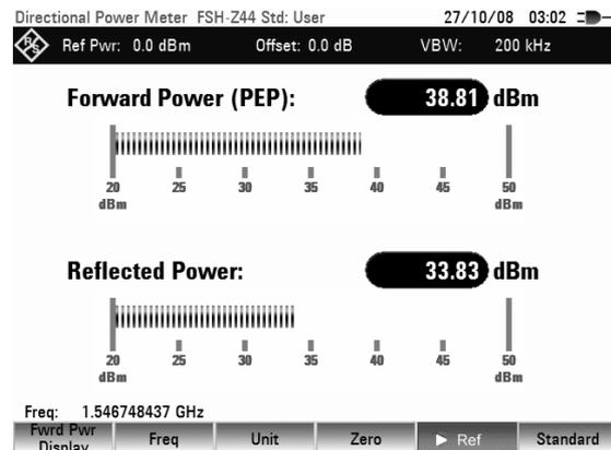
To ensure that true results are output when measuring modulated signals, the R&S FSH offers the possibility of taking correction values into account for a number of common transmission standards.
