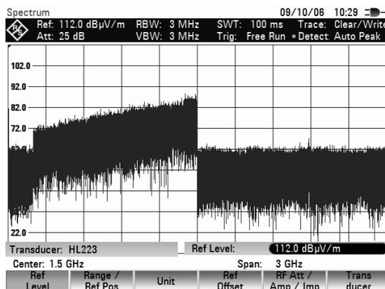
A second transducer factor can be selected with the SELECT SECONDARY TRANSDUCER softkey, which is then added to the first, as soon as the menu entry [ ] SELECT SECONDARY TRANSDUCER is marked with an X. The unit of the second transducer factor must always be the relative unit dB as otherwise an addition would not be useful. When SELECT SECONDARY TRANSDUCER is selected, the R&S FSH offers only the transducer factors stored in the instrument with dB as the unit.
