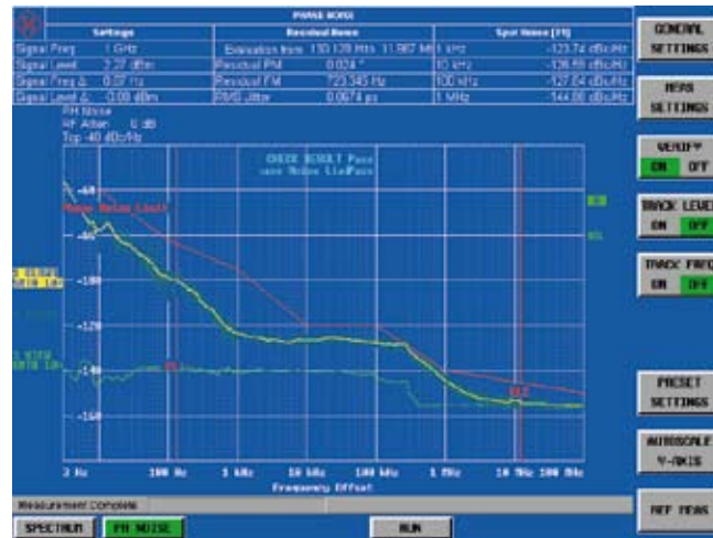
Phase noise measurement using the R&S®FS-K40 Application Firmware.
