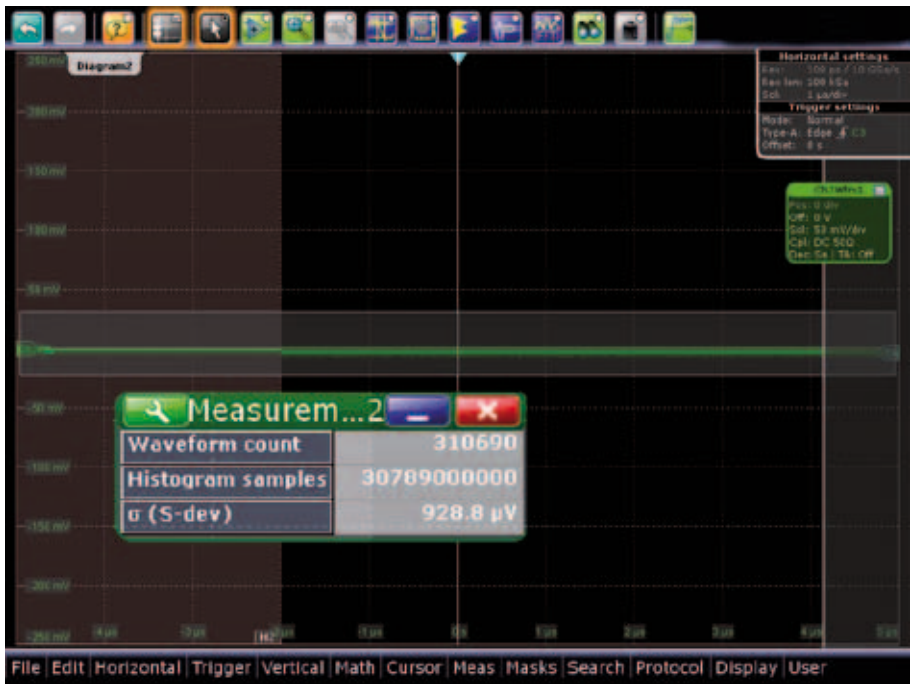
Typical inherent noise of the R&S®RTO1024 oscilloscope: standard deviation (S-dev) with histogram measurement. Measurement conditions: 50 mV/div, resolution 100 ps, no filter.
