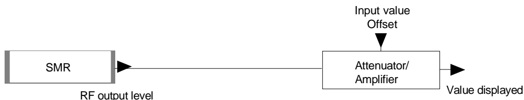
Fig. 4-4 Typical setup with level offset
