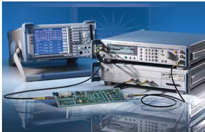
Module test with the R&S®SMV03, R&S®AMIQ and Spectrum Analyzer R&S®FSP
