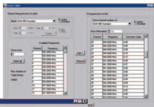
Path characterization wizard: definition of frequency ranges for a scan
