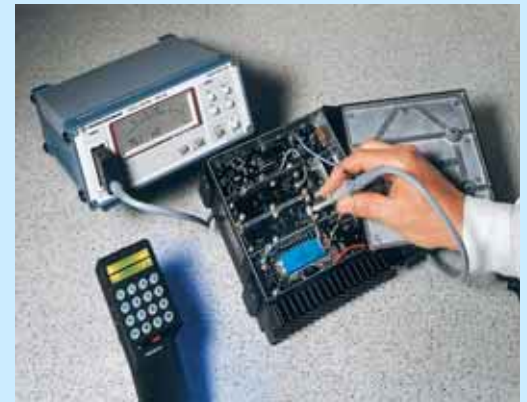
Low-load voltage measurement with the RF Probe R&S®URV5-Z7
