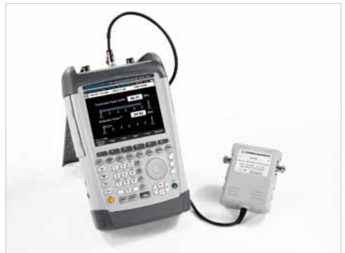
The R&S ZVH with directional power sensor.
