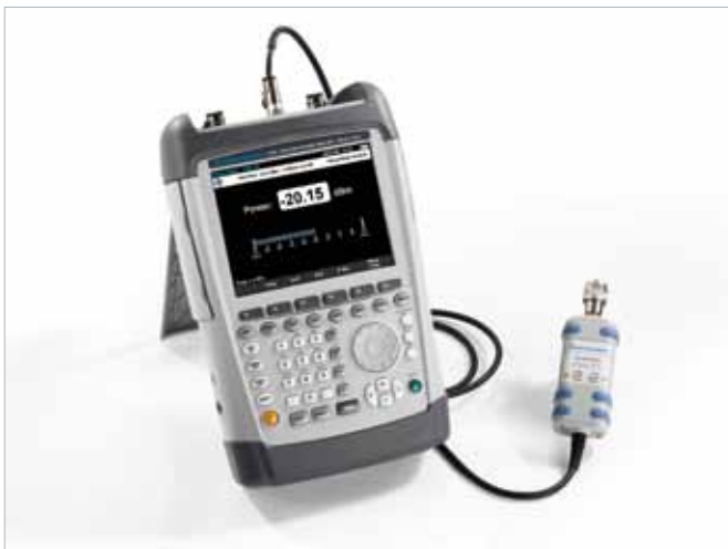
The R&S ZVH with terminating power sensor.
