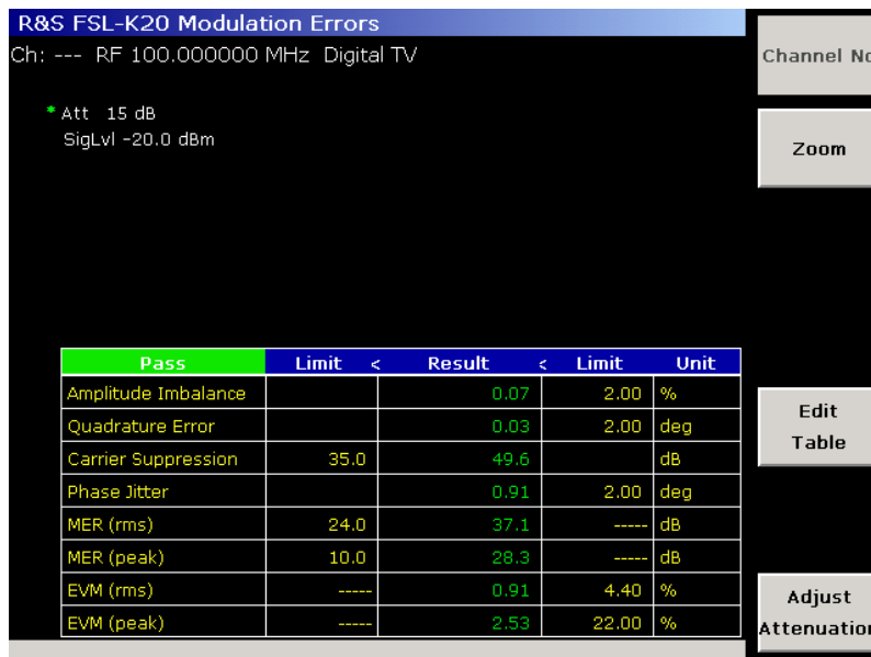
Fig. 2-55 Digital TV Modulation Errors measurement
