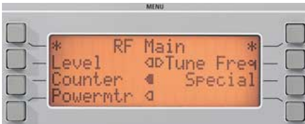
Softkeys enable fast access to measurement functions
