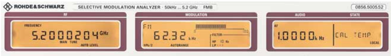
All important test parameters are indicated simultaneously on clearly arranged LCDs
