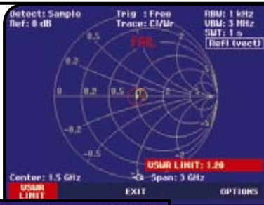
Measurement of magnitude and phase in Smith chart
