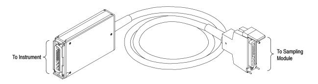
**3.** Use the connector marked "To Sampling Module" to connect to the sampling module. See the sampling-module user manual if you require information on connecting signals to the sampling module.
