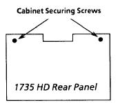
Figure 1–5: Cabinet securing screws
