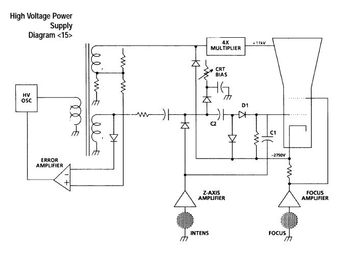
The High Voltage Power Supply generates the heater, cathode, control grid, focus anode, and post accelerating potentials required to display the outputs of the Vertical and Horizontal Output Amplifiers.
