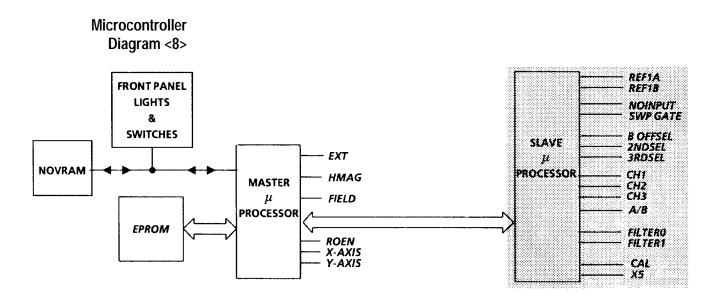
**Master Processor.** The master processor consists of U33 and U32. U32 is the erasable-programmable read-only memory (EPROM) containing the instruction code for the microprocessor, U33. Port 0 of U33 is used for multiplexed address and data lines. U31 is a tri-state octal D-Type latch which determines the address lines. The front-panel switch matrix is read directly by U33 through Port 1 which provides a stimulus via ROW 0–3, and evaluates the response through COL 0–3.
