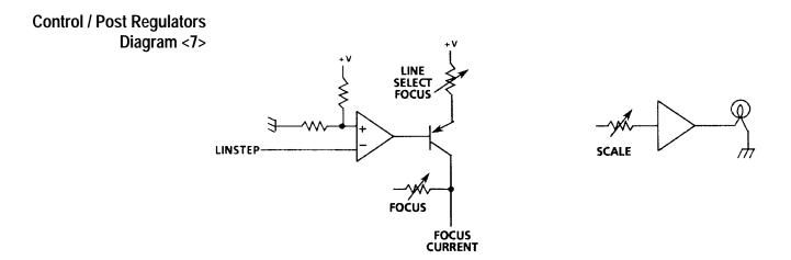
**Focus Amplifier.** The FOCUS control affects two different display modes; normal mode and LINE SELECT mode. In the normal mode of operation, the focus voltage will be selected by the control setting only (Q1). When a LINE SELECT (LINSTEP) pulse occurs, U3A turns off and additional current flows through Q1. The LINE SELECT FOCUS adjustment (R6) is adjusted for optimum focus while operating in LINE SELECT mode at the normal display focus setting.
