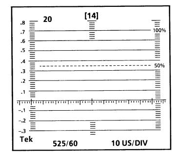
Figure 2–13: 1735 HD on-screen readout for line-select operation, with 14-line selected
