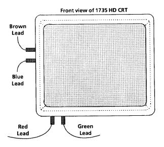
Figure 7–5: Positions of CRT deflection leads
