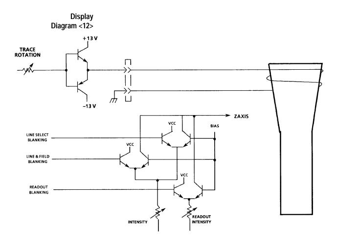
**Trace Rotate.** Trace rotation is necessary to compensate for changes in the magnetic field surrounding the 1735 HD. Q18 and Q19 are emitter followers that provide the trace rotation current to a coil located inside the CRT shield, around the tube. Current amplitude and polarity are controlled by the front-panel ROTATE screwdriver adjustment.
