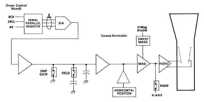
**Sweep Generator.** The sweep generator is controlled by the microcontroller. Sweep and retrace are directly enabled and disabled by the control line /SWPGATE, which is high for retrace and low for sweep. If Q16 is off, the sweep ramps up at a rate determined by the current from the DAC (U17) and the timing capacitor (C63 for line rate sweeps or C63 with C62 in parallel for field rate sweeps).
