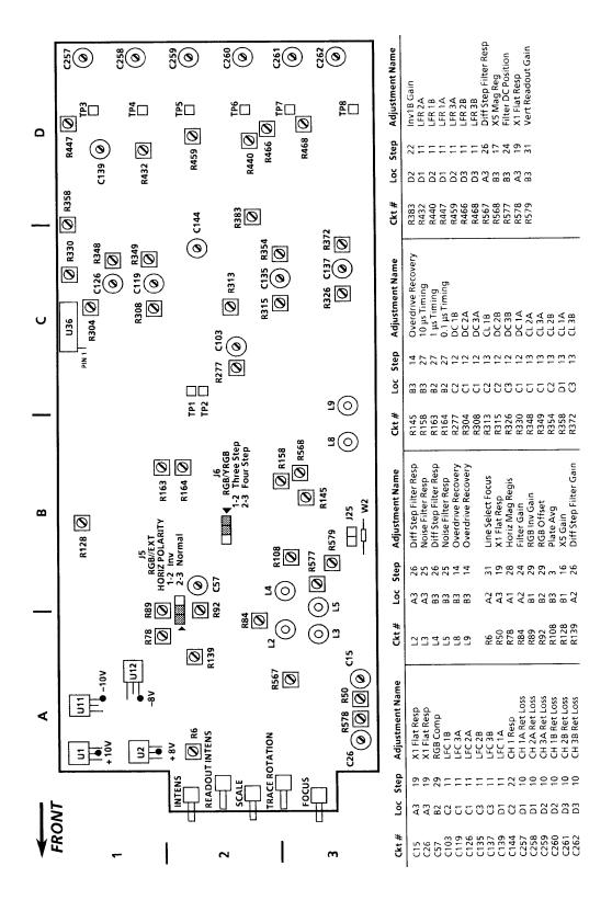
Figure 6–2: Adjustment locations on the Main circuit board (Assembly A3)
