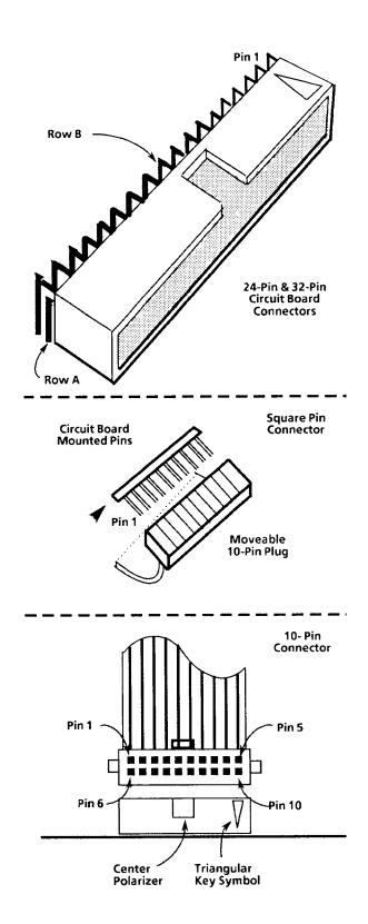
Figure 7–3: Multiple pin connectors
