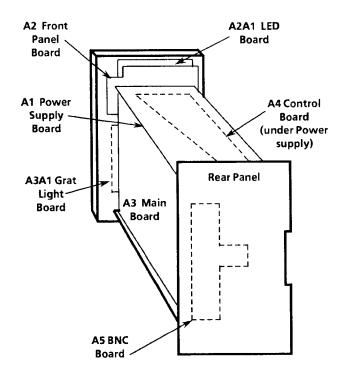
Figure 7–2: Circuit board assembly locations
