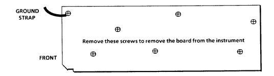
Figure 7–9: Screws that hold the Power Supply board (A1) in place
