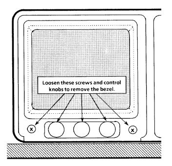
Figure 7–4: Bezel screws
