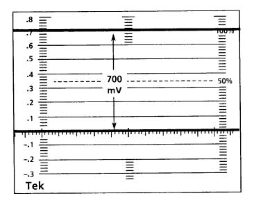
Figure 2–9: 1735 HD calibrator signal
