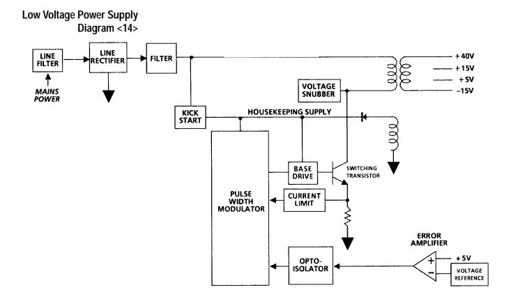
The low voltage power supply converts the mains line voltage (between 90 and 250 volts) to supply the power requirements of the instrument. The low voltages supplied from the central power supply are +40 V, +15 V, +5 V, and -15 V.
