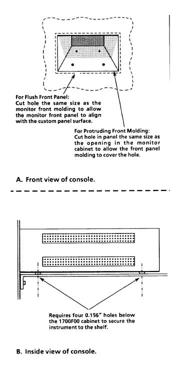
Figure 1–9: Typical custom installation
