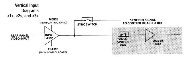
**Inputs**. Each of the six video input channels of the 1735 HD has an identical video input amplifier. These channels are arranged in two groups of three each (1A-2A-3A and 1B-2B-3B). CH 1A circuit numbers are used here.
