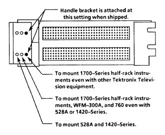
Figure 1–7: 1700F05 Rack Adapter adjustment
