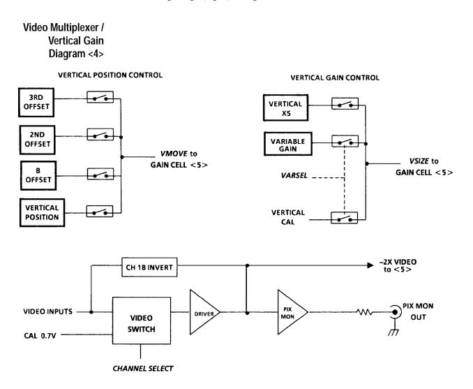
**Video Switch and Pix Mon.** Multiplexer U50 selects a signal from one of its eight video inputs, controlled by the three select signals VMUX0, VMUX1, and VMUX2. The video switch has unity gain. The driver gain is 1.78, and the video gain from the rear panel to the driver output (U38, pin 6) is approximately 2.
