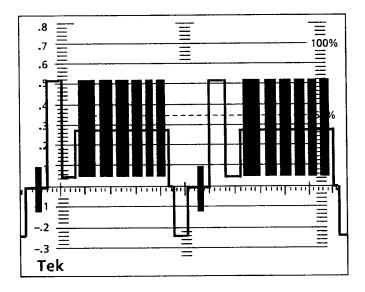
Figure 2–11: Multiburst signal; two-line flat display
