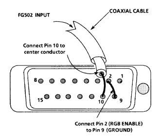
Figure 5–1: REMOTE connector modified to check RGB operation
