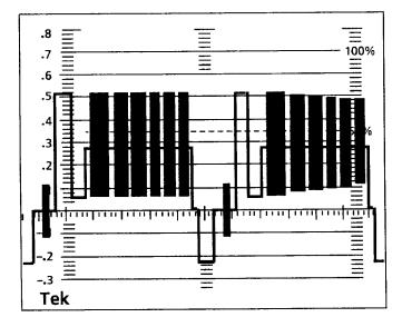
Figure 2–12: Multiburst signal; alternate lines filtered and flat
