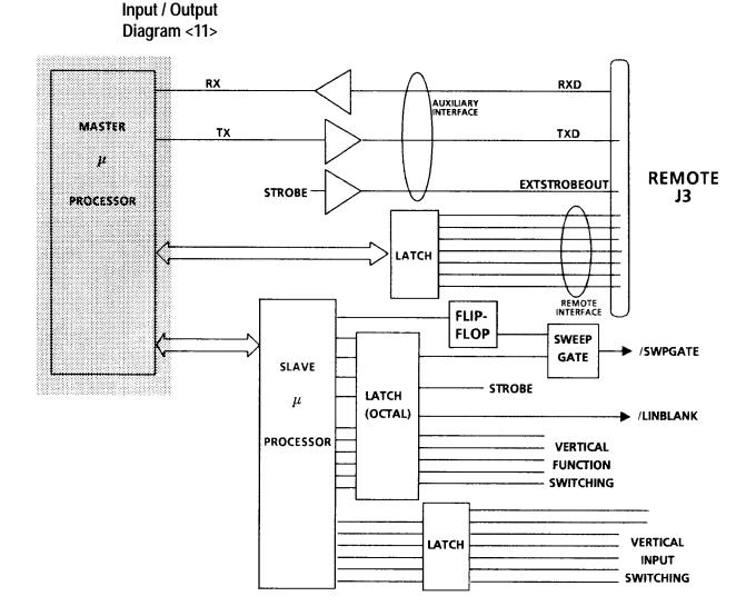
**Master Slave Interface**. The slave microprocessor (U11) acts as the main link between the master microprocessor and the hardware of the instrument. Constant serial communications between the processors keep the slave informed of any front panel changes. The slave then configures the instrument hardware to produce the correct display. The slave is also responsible for handling line counting in LINE SELECT mode.
