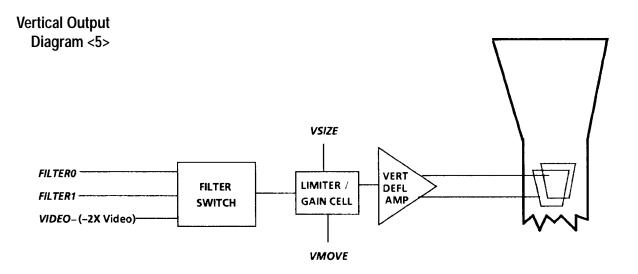
**Filter Select.** When no filter is selected (FLAT), full bandwidth video passes through U10 to the gain cell in U25; U15 and U9 are disabled. When the NOISE filter is selected, filtered video passes through U15 to the gain cell in U25; U10 and U9 are disabled. When the DIFF STEP filter is selected, filtered video passes through U9 to U25.
