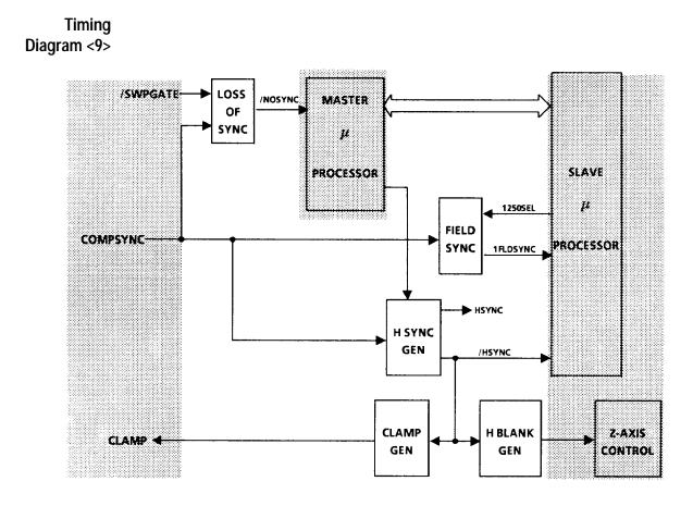
**Horizontal Sync Generator.** The horizontal sync generator produces a pulse that starts just before sync and ends at the leading edge of sync. Since the 1735 HD is a multi-standard instrument, the time from the leading edge of sync to the start of the pulse is programmable and controlled by U33 (Diagram 8). The ramp starts up at the leading edge of sync. A voltage comparator determines when the HSYNC pulse starts and the ramp resets.
