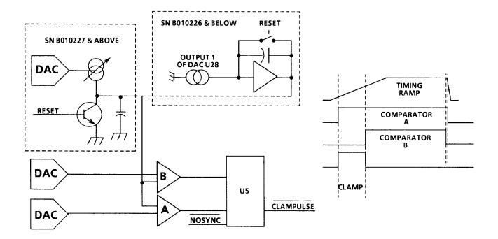
Figure 4–2: 1735 HD Clamp pulse generator
