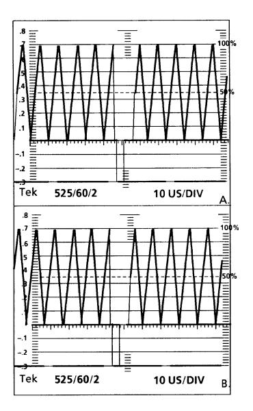
Figure 5-3: Checking horizontal timing
