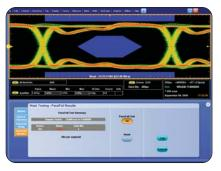
► Testing a 622 Mb/s signal against the mask specified by the standard.
