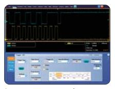
► Easily trigger on a specific I<sup>2</sup>C address.
