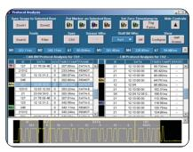
► CAN and LIN Timing and Protocol Decode.
