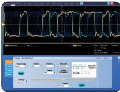
► Serial pattern triggering to debug pattern-dependent issues.
