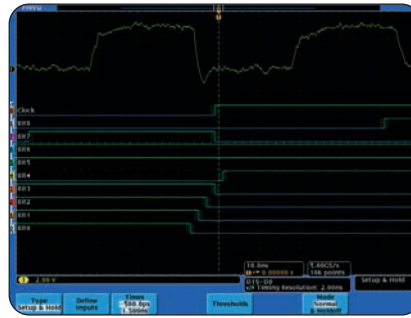
► Multi-channel setup-and-hold triggering highlighting multiple violations (MSO4000).
