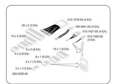
34-channel Probe Interface Kit with mini-PV Connectors.
