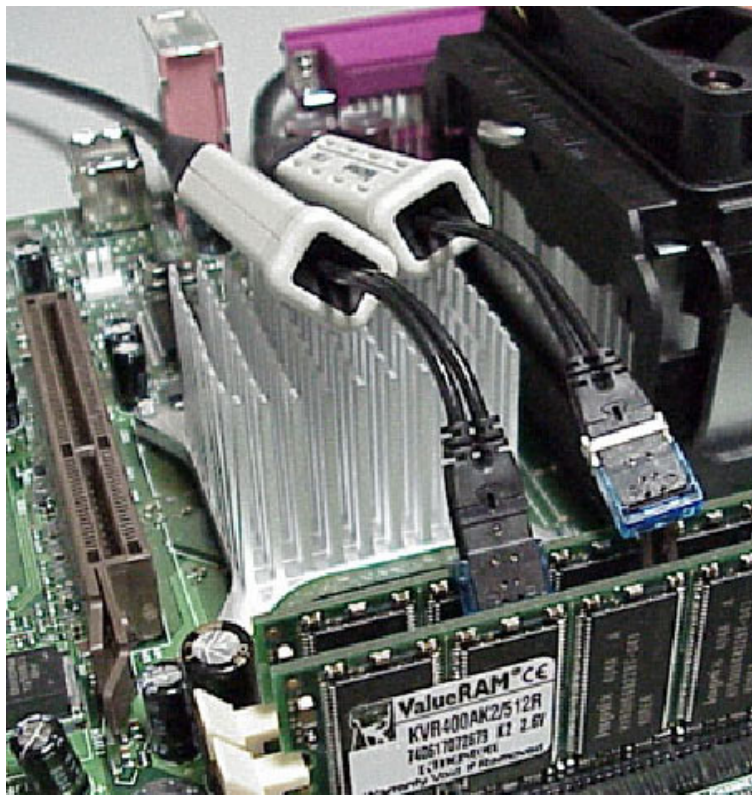
Figure 10: Soldered Tip-Clip assemblies
