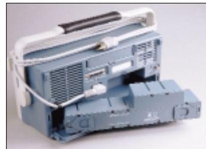
TDS 3BAT – Battery Pack being installed.
