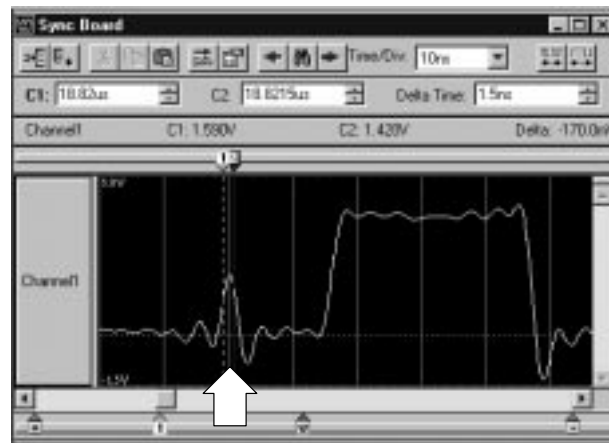
Figure 2-17: DSO module triggering on a glitch
