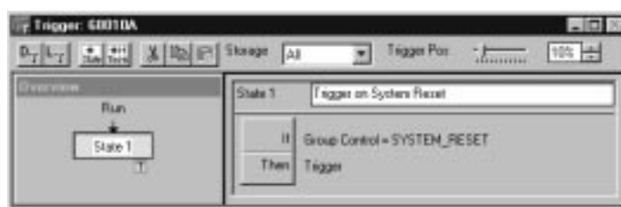
Figure 2–21: Using symbols in a trigger program
