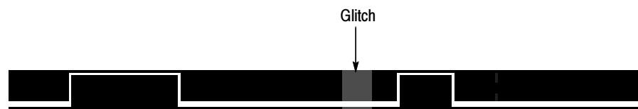
Figure 3- 80: Waveform with a glitch
