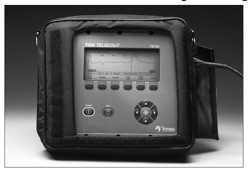
If your job is to find faults on telephone twisted pair cable, the Tektronix TelScout™ TS100 is built for you. Designed specifically for telephone local loop applications, the TS100 applies the newest technology to provide both ease of use and telephony performance that cannot be found in any other TDR.
