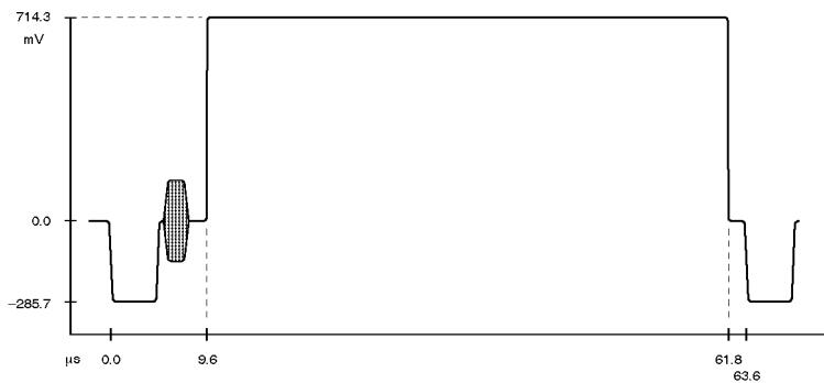
Figure 33: NTSC 100 IRE Flat Field, Field Square Wave, and Bounce (High)
