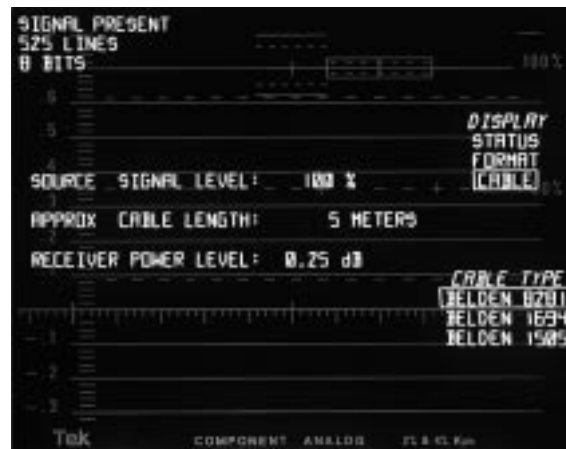
The WFM601E and WFM601M provide a display of important data signal analog parameters.
