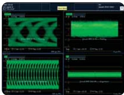
► Figure 11. 3-Eye, 20-Eye and jitter waveform.
