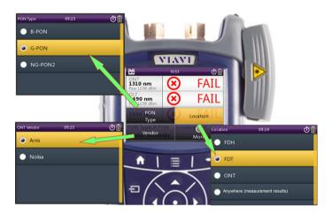
Easily select PON-type, Location, and Vendor to setup standard pass/fail thresholds providing reliable acceptance testing with simultaneous display of all PON and video power levels.
