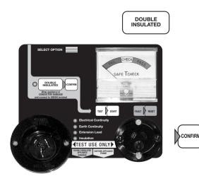
8 Confirm the connection of the conductive bandage wrapped around the appliance under test to the **SAFETCHECK MKD** by pressing the confirm membrane pad.
