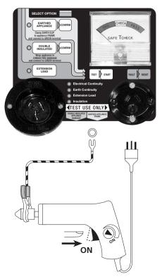
If any earthed appliance has one or more metal component(s) which are possibly not connected together, the overall test must be repeated with the EARTH clamp connected to each metal component in turn.
