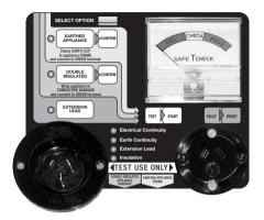
Place **SAFE7CHECK MKD** on a convenient nonconductive working surface. Plug the power cord into **SAFE7CHECK MKD** receptical at the rear of the unit and connect plug to the 240V 50Hz supply. Switch the 240V 50Hz supply 'ON'.
