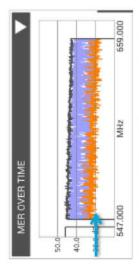
Unstable MER with drops below 30dB means only profiles running 256 QAM or lower will work.
