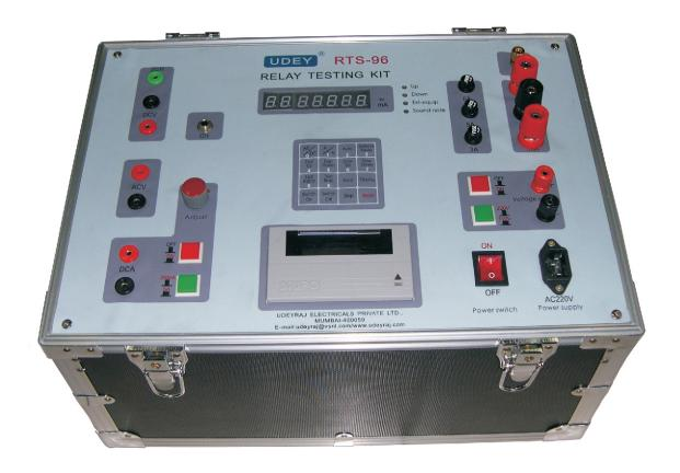
**Introduction:** Model 'RTS-963' is an ideal, newly developed multifunction relay tester adopting monolithic computer technology. It is composed of auto synchronized digital millisecond timer, logic controlling unit, multifunction digital display, high precision digit collection and processing unit, current-voltage output unit, overload and over range protection unit. Test process is automatic for improved efficiency. The tester has a built in printer for printing the results.
