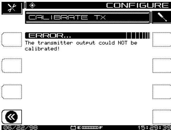
Fig. 2-13 Calibrate Error (Missing Jumper Cable)
