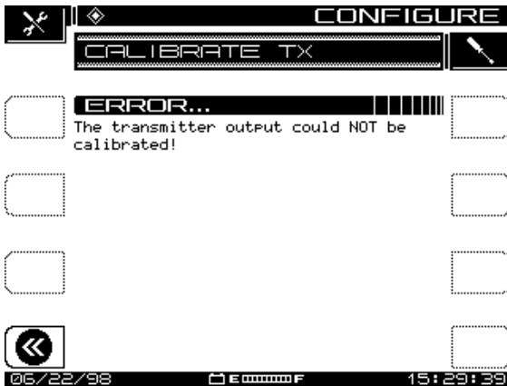
Fig. 2-13 Calibrate Error (Missing Jumper Cable)
