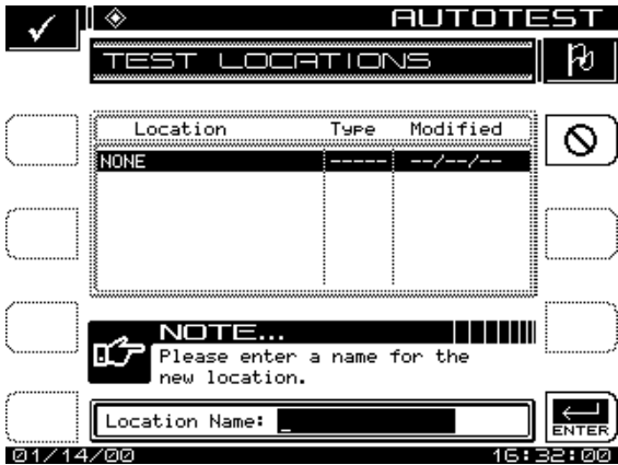
Fig. 13-25 Naming a Test Location
