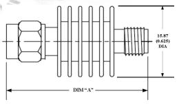
**Construction:** Black aluminum alloy body with passivated stainless steel connectors. Gold plated beryllium copper contacts.
