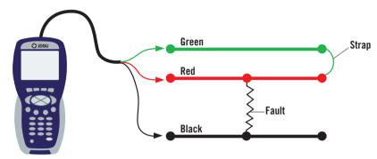
It is important to note that RFL testing takes approximately 30 to 40 seconds. Arrows indicating the paths that are being tested will be displayed on the HST-3000's screen. Once the test is completed, each result will be shown in either ohms or feet.
