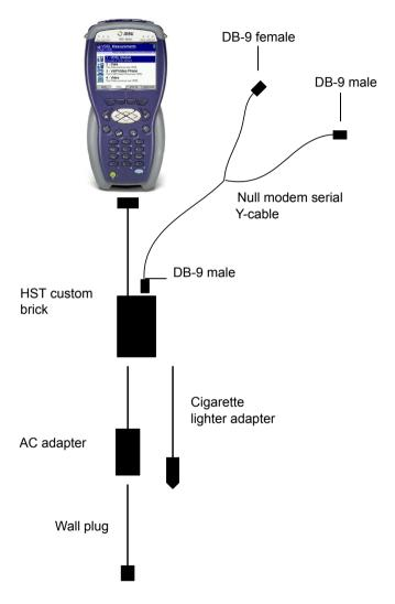
Figure 13 VT100 power cabling option with a 14pin battery
