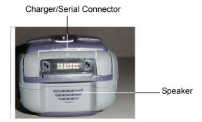
Figure 6 HST-3000 bottom panel with 14pin battery
