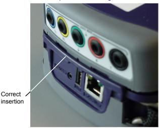
Figure 9 Inserting the SIM tab
