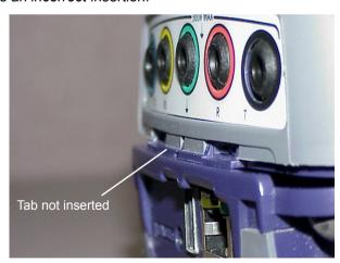
Figure 10 Incorrect SIM attachment
