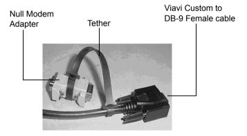
Figure 11 VT100 standard cabling
