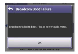
If the meter is showing this error, the issue could be caused by software or hardware failure.
