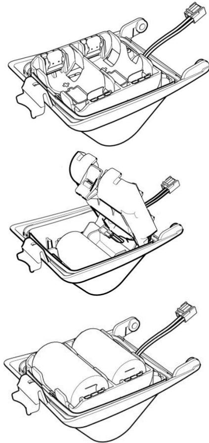
**Figure 3.4 Locator D-cell holder**
