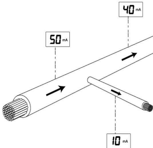
Figure 6.3 Current readings
