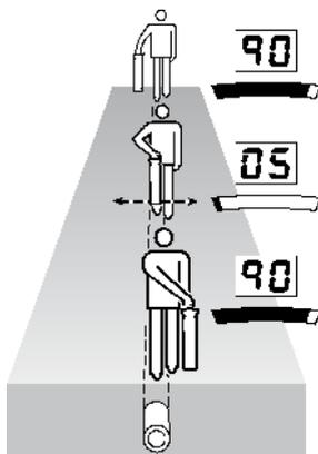
Figure 4.1: Line Tracing
