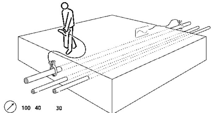
Figure 8.1: Connecting clamps
