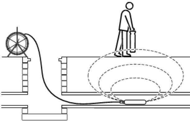
Figure 8.7 Sonde deployment
