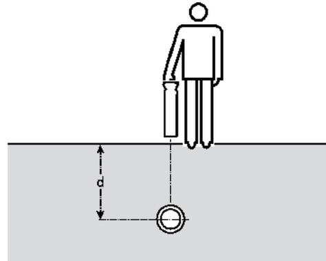
Figure 6.1: Taking a depth reading
