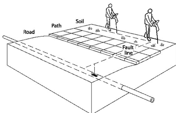
**Figure 9.2: Locating faults with the locator and A-frame**
