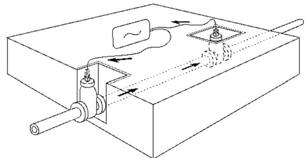
Figure 8.5: Making double-ended connections
