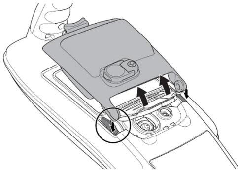
**Figure 4.6 installing a new battery pack**
