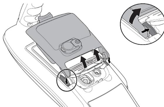
Figure 4.4 Press the retaining latch inwards
