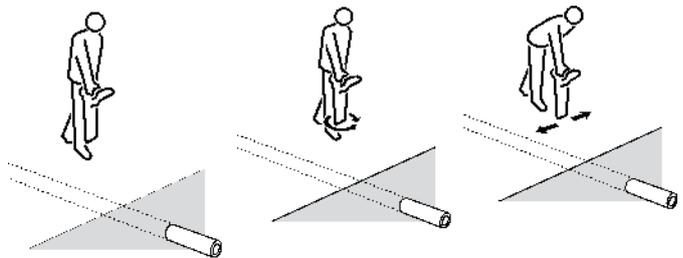
Figure 5.6: Pinpointing a target line
