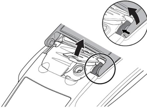
**Figure 4.5 Repeat then lift the battery pack away**
