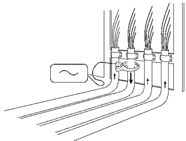
Figures 12.4 – 12.5: Connecting transmitter clamps
