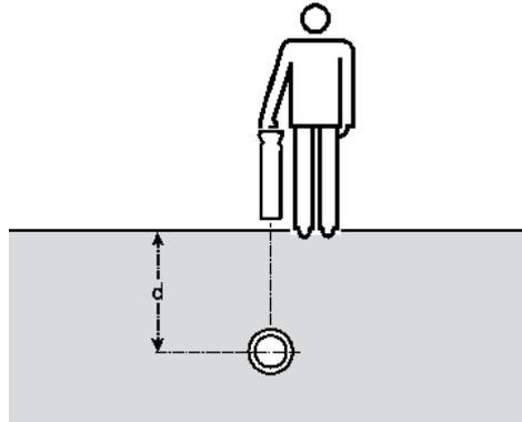
Figure 7.1: Taking a depth reading
