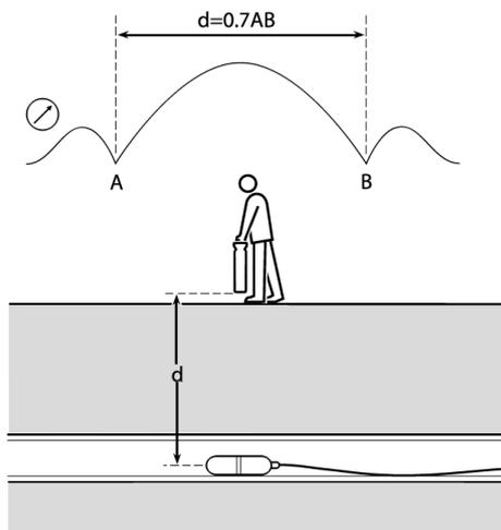
Figure 12.8: Calculating sonde depth
