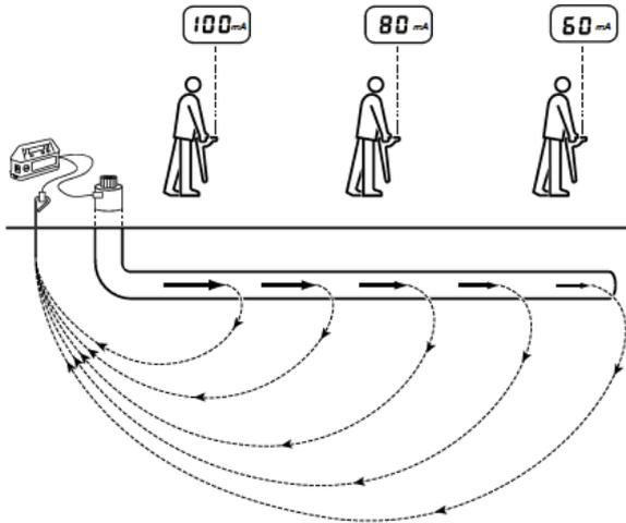
Figure 7.7: Current readings using transmitter signals
