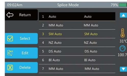
← Enter into the splicing mode and select and press the needed one (yellow font is the current splicing mode).
