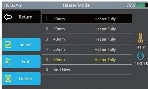
Enter into [Heater Menu], choose the needed mode, then press until the font become yellow; this is the current splicing mode.
