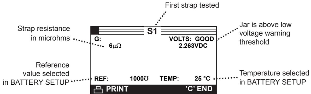
**\*\* NOTE:** The analyzer displays and prints dashes (-----) if you selected VOLTS ONLY in BATTERY SETUP, or if you selected VOLTS THEN CONDUCTANCE, but did not complete the conductance measurement.
