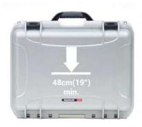
ASTM D-4169 DC-18 DROP TEST
