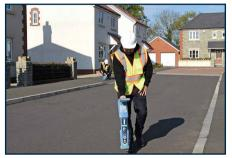
A locator for all industries 7 active and 4 sonde frequencies, 3 passive modes, power filters and other advanced features to provide efficient accuracy for locating and tracing burried utilities.
