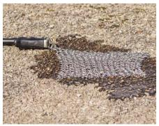
Simply lay the Earth Mat out flat on the ground and connect the Transmitter or Genny Earth Lead. Pour a little water on the Earth Mat for an improved signal and start scanning immediately – more quickly and more easily than ever before.
