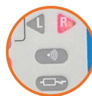
Rotary Field Indication, Continuity & Low Impedance
